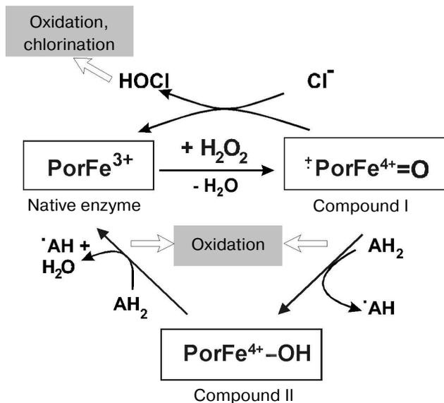
**Fig. 1.** Halogenation and peroxidase cycles of myeloperoxidase. Both cycles utilize hydrogen peroxide to oxidize the native enzyme to compound I. Por denotes porphyrin.  $\text{AH}_2$  and  $\cdot\text{AH}$  represent substrates being oxidized and the formed radical product, respectively. Instead of  $\text{Cl}^-$  other (pseudo)halides such as  $\text{Br}^-$ ,  $\text{I}^-$ , and  $\text{SCN}^-$  will also be oxidized by compound I. Other pathways of myeloperoxidase are only denoted.
